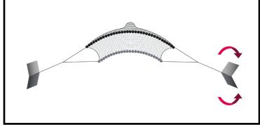
Depth sensors indicate the distance from the surface to the doors/trawl.
