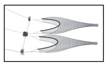
For twin and multi-rigging vessels, the spread on EACH net is provided. This allows for equal bulk in EACH net.
