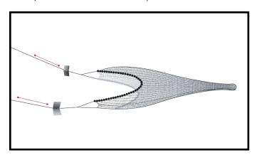
Major fuel savings are achieved with doorspread by adjusting the speed of the vessel to keep the optimal spread. For example, towing just 0.1 knots too fast into a current can overspread the gear by 10 meters.
